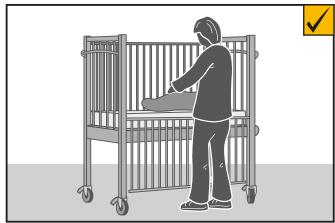
Cot is designed with a higher working height, reducing the workers need to reach and bend to lift children into/from the cot.
