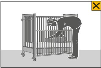
Cot base is non-adjustable and close to the ground, requiring workers to reach and bend to lift children into/from the cot.
