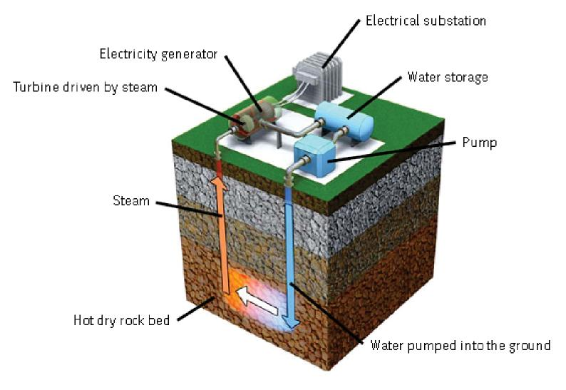
We have learnt scientists have built geo thermal plants that use the Earth's hot core to heat water. The hot water turns to steam after going deep in the earth. The steam turns the electrical generator.
