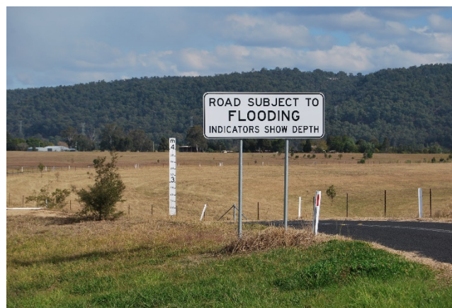
Flood sign and depth indicator in the Penrith / Emu Plains floodplain of the Hawkesbury-Nepean Valley showing inundation levels.
