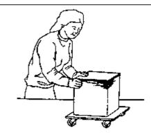
Figure 44 - Rolling platform to avoid lifting
