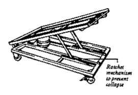
Figure 45 - Rolling platform with tilt mechanism
