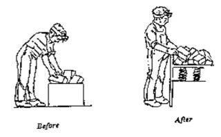
Figure 10 - Raise work level by use of self-adjusting platform
