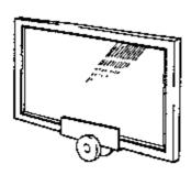
Figure 36 - Wheel set enables pushing in place of lifting
