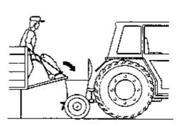
Figure 19 - Gravity feed principle to avoid lowering
