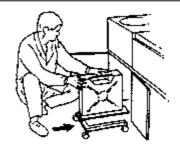
Figure 27 - Simple trolley avoids awkward handling
