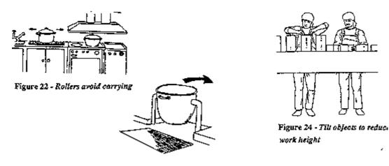
Figure 23 - Pour without lifting
