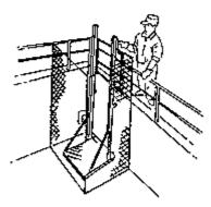
Figure 61 - Elevator for transporting goods between floors
