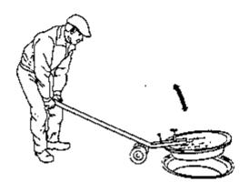
Figure 42 - Levers reduce force required
