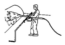
Figure 30 - Use structures to absorb reaction forces
