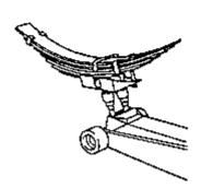
Figure 34 - Support weight by use of Jack
