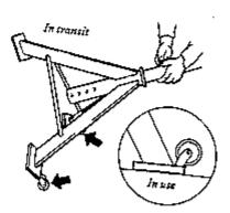
Figure 38 - Wheels avoid carrying when moving
